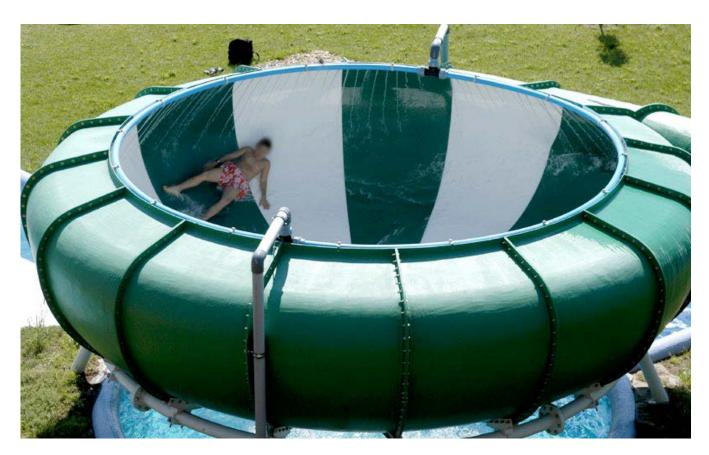
An untypical slide of a specific structure: created for aqua parks. The whole slide is divided in three stages: 1/gathering speed stage in the relatively long and steep section, which is made of 800 mm tube; 2/ repeated centrifugal rotation in the onion-shaped bowl; 3/ free fall to the pool below or, alternatively, end of slide at the tube stage. Similar to its bigger counterpart Space Bowl 6500, it is possible to combine it with the other slide or pool.
