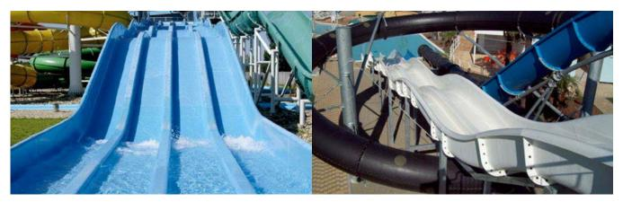
As the name suggests, this construction is composed of many tracks parallel and connected to each other, which allows several people to slide simultaneously with no risk of collision. Additional attraction related to the slide is a possibility of friendly competition between the users. The slide is available in options 2,3,4 and 5-track, and more than that, it allows to use tracks from 2 to 5 at the same time.
